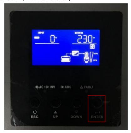
(c) Press 'Up' and 'Down' to choose the setting item No., press 'Enter' to enter into the detailed setting parameter, when finish press 'Enter' again. The following setting items need to be set follow the recommended value:
